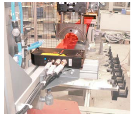
Bearing shell detection in automotive manufacturing
